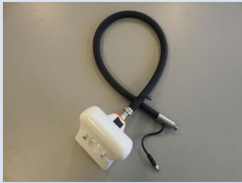
Mouthpiece Handheld with heatable Transferline
